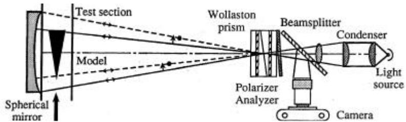
Fig.2. Experimental set up modified for axisymmetric flows
