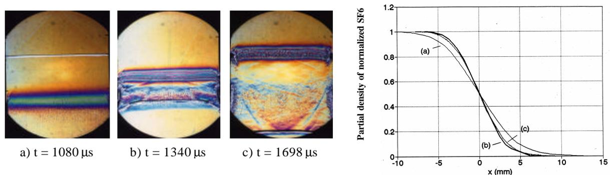
Fig. 4. Gas density profiles of SF<sub>6</sub> - Interface: SF<sub>6</sub> – Air , Ms = 1.45
